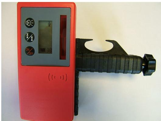
Fit the supplied 9V battery, polarity marked. Power up - via red ON/OFF button.
