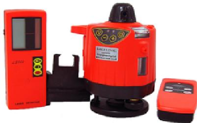
Fit the supplied 9V battery, polarity marked. Power up - via red ON/OFF button. The middle button sets either **coarse** (+/-2mm) or **fine** (+/-1mm) pick-up window resolution.
