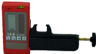
Fit the supplied 9V battery, polarity marked. Power up - via red ON/OFF button. The next button sets coarse (+/-2mm) or fine (+/-1mm) pick-up resolution. The User can switch the sounder to High / Low volume or OFF, as required. The far right-hand button controls a display back-light for use in low lighting conditions on site.
